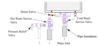
For increased energy efficiency, use pipe insulation. Please install the insulation according to the diagram above, making sure to insulate all the way to the top. **Do not** cover any drain or pressure relief valve(s).
